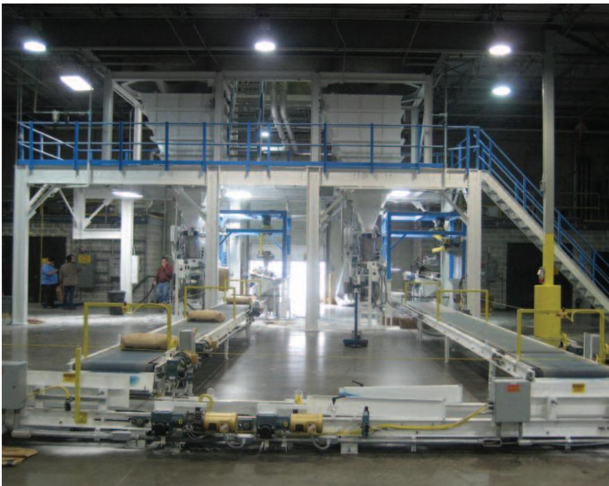
***The two parallel packaging lines consistently fill up to 24 bags per minute, exceeding the company’s original packaging rate requirements.***
